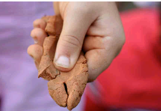
FIGURE 1. To make a soil ribbon, moisten your soil and then push it across your pointer finger with your thumb. How long is it?
