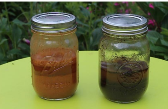
FIGURE 1. One jar is a clayey soil still settling and the other is a loamy sand.
