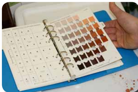
The Munsell Color Chart allows soil color to be quantitatively measured.
